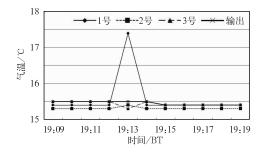
图 10 1 号温度传感器气温异常 Fig. 10 The abnormal data of No. 1 temperature sensor
