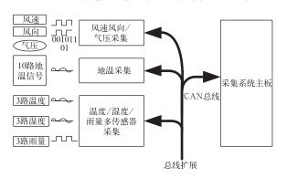
图 1 同一要素多传感器硬件系统结构 Fig. 1 System structure of multi-sensor automatic weather station
