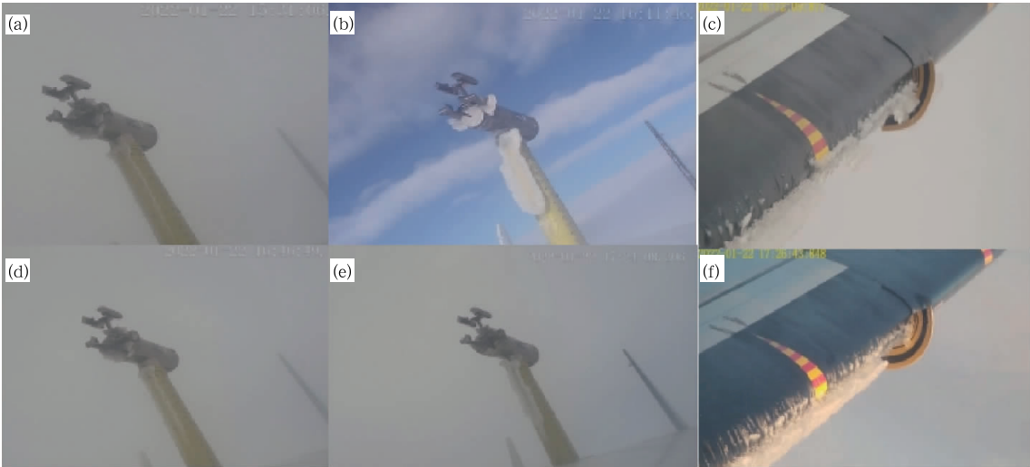
图 2 2022 年 1 月 22 日自然结冰取证试飞过程飞机结冰图像 (a)15:31 第 1 次云中,(b)16:11 第 1 次出云,(d)16:46 第 2 次云中,(e)17:24 第 2 次出云 CCP 热线含水量电路板结冰状态;(c)16:12 第 1 次出云和(f)17:26 第 2 次出云后左侧机翼 2 号标尺结冰状态 Fig. 2 Aircraft icing during the natural icing certification flight test on 22 January 2022 (a, b, d, e) the circuit board icing condition of CCP Hotwire of (a) the 1st time in cloud at 15:31 BT, (b) the 1st time out of cloud at 16:11 BT, (d) the 2nd time in cloud at 16:46 BT, (e) the 2nd time out of cloud at 17:24 BT; (c, f) the No. 2 ruler icing condition of left wing after (c) the 1st time out of cloud at 16:12 BT and (f) the 2nd time out of cloud at 17:26 BT
